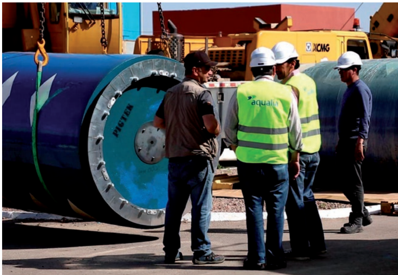
PIG technology applied for cleaning water intake pipes in the Mostaganem, Algeria, desalination plant.
