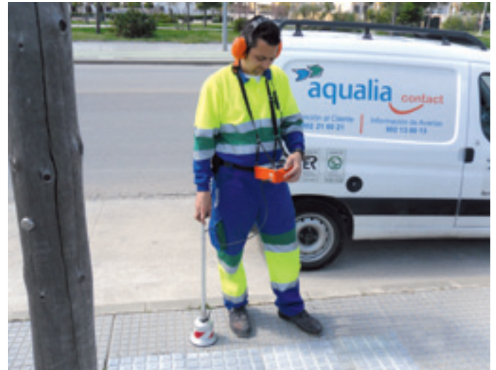
FCC Aqualia personnel performing leak-detection tasks.
