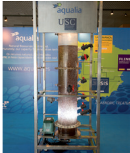
Sample of the Anammox technology pilot developed in partnership with the University of Santiago de Compostela at the AD13 Congress.
