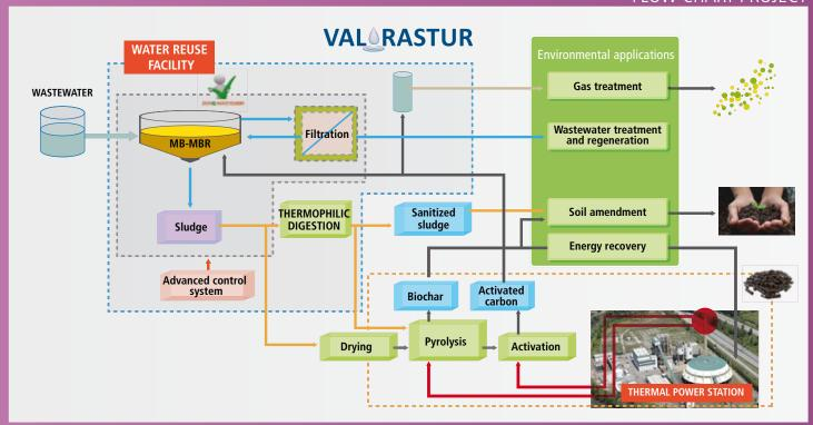
The dry and sanitized biosolids resulted from the proposed advanced sewage sludge treatment show characteristics that make them suitable to be used as fuels in the thermal power plants (HUNOSA, partner in VALORASTUR project). With this aim, the drying process and the combustion conditions of dry sewage sludge will be optimized. Furthermore, gaseous
