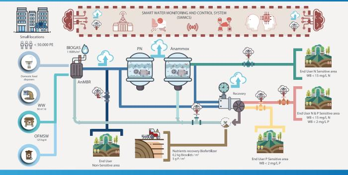
The project will also be equipped with a smart water monitoring and control system (SWMC) which will allow obtaining different types of water quality depending on the legal requirement and the needs of the end user.
